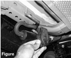
Driver side rear hanger: Once you have removed lower pin from the grommet, continue to remove the arommet.
