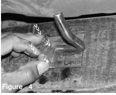
The two m8 bolts in this kit are used to secure the bracket in place.
