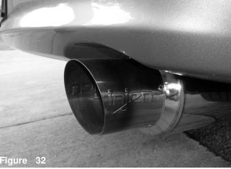
Rear muffler with signature series, titanium tip.
