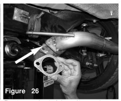
The 60mm metal gasket is inserted between the rear muffler flange and the secondary mid-section flange.
