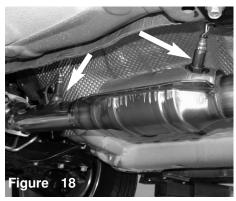
Both O2 sensor bungs are now fully fastened to the primary pipe with the catalytic converter.
