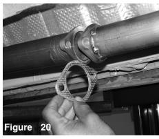
Place an oval metal gasket between the primary and secondary pipe. Use two m10 bolts and flange nuts to secure the two ends together.
