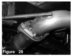
The m10 nuts and bolts are tightened just enough to hold the two flanges together.
