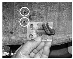
New bracket is aligned to the rear cross member.
