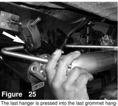
The last hanger is pressed into the last grommet hang ing on the bracket installed earlier.
