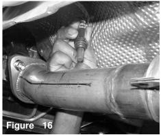
The first 02 sensor is inserted into the sensor bung located on the primary pipe.
