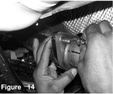
Use two m10 bolts and flange nuts to connect the test pipe and the primary section together.
