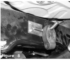
The grommet is placed over the new bracket as shown above.
