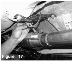
The secondary O2 sensor is placed into the catalytic converter sensor bung.
