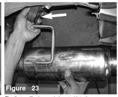
The first muffler hanger is inserted into the rear grommet
