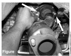
Tension bolts are removed from the primary catalytic converter. Once you have removed the tension bolts continue to pull the catalytic converter.
