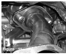
The stock tension bolts are used to fasten the test pipe in place,
