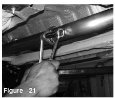
A 14mm socket and ratchet are used to tighten the nuts and bolts together.
