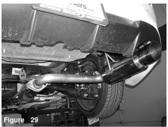
Side shot of the installed rear muffler section.
