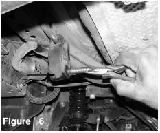
Driver side rear hanger: Grommet pin is removed from the grommet. The grommet is then pulled from the metal hanger.
