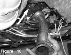
The new test pipe is aligned to the header exhaust as shown above.
