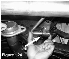
The inside hanger on the exhaust pipe is pressed into the second grommet.
