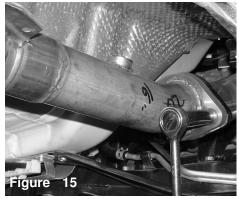
A 14mm socket and ratchet is used to tighten the two m10 bolts.
