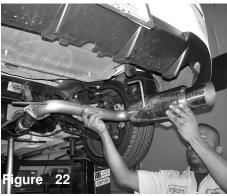
The rear muffler is now aligned to the end of the secondary pipe, while aligning the three hangers to the stock grommets.
