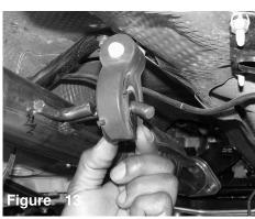
The primary section hanger is inserted into the stock grommet.
