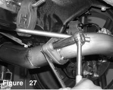
A 14mm socket and ratchet is used to tighten the nuts and bolts together.
