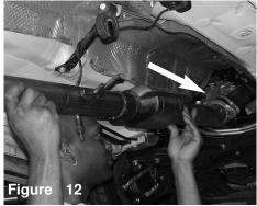
the primary section with the catalytic converter is aligned to the test pipe.
