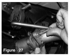
Two m10 bolts and nuts are used to secure the two flanges together.
