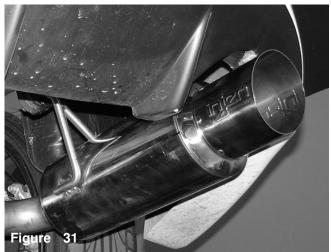
Inside shot of the installed rear muffler section.
