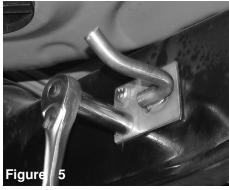
Use a socket and ratchet to tighten the bolts in place.
