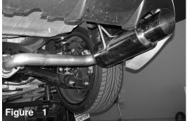
60mm high flowing exhaust system with catalytic converter, titanium tip and test pipe.
