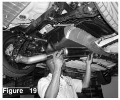
The secondary pipe is now aligned and connected to end of the primary pipe with the catalytic converter.
