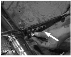
install the hangar bracket assembly to the exhaust using provided M8 screws. *Do not tighten.*
