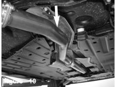
Now install the mid-pipe to the exhaust. Secure using provided 3" gasket and bolts with nuts. *Do not tighten.*
