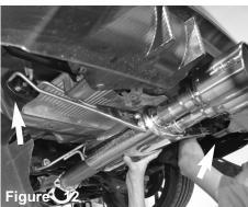
Position all the hangars to to the isolation mounts. (*look for UP sign on mount*) Position and adjust fitment. *Do not tighten*.
