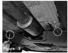
Loosen the screws holding in the factory engine cover. This will allow to loosen screws on pipe.
