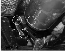
Loosen the 3 nuts holding in the pipe using 14 mm socket with wrench. Save these 3 nuts for later install.
