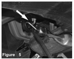
Pull back the rear covers allowing for access to the rear hagnars. With lubrication, remove all the exhaust hangars from the rubber isolation mounts.
