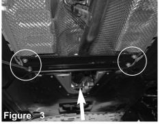
Loosen the screws holding in the factory engine cover. This will allow to loosen screws on pipe. Loosen and remove the lower strut brace.
