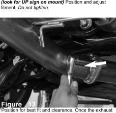
is in correct position, Secure and tighten. Secure the bracket assembly also. Note: Exhaust system has room for adjustment, re-position and tighten for best fit.
