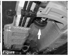
Remove the isolation mount from the exhaust closest to the 3 hole flange. Re-install to the vehicle. Make sure the isolation is facing in the correct direction. (look for UP sign on mount)
