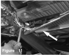
install the hangar bracket assembly to the exhaust using provided M8 screws. Snug fit with allen key, do not tighten completely.
