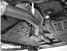
Now install the mid-pipe to the exhaust. Secure using provided 3" gasket and bolts with nuts. Do not tighten.
