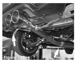
Position all the hangars to to the isolation mounts. (look for UP sign on mount) Position and adjust
