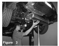
Remove the entire stock exhaust from the Catalytic converter.
