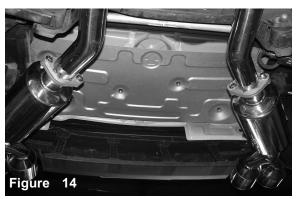
Rear muffler section secured to mid-pipe sections. Make your final adjustment and make sure you have clearance with no iterference with the bumper or chassis components. you may now Tighten all the bolts supplied once all adjustment have been made and then recheck again.
