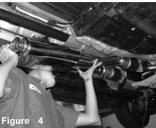
Install the midsection with the two tubes attached to it to the factory catalytic converters.
