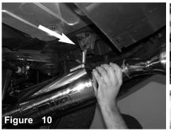
Take the passenger side rear muffler section hanger and insert it into the rear exhuast grommet.
