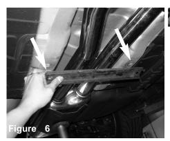
Loosen the two 10mm bolt and remove the mid section bracket. This bracket will not be reused in this install. You may re-insall the two 10mm bolts to secure the heatshield
