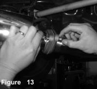
After the gasket is in place. Insert two M10 bolts with nuts to secure the flanges together on both drivers side and passenger side. Leave these nuts and bolts loose for now.
