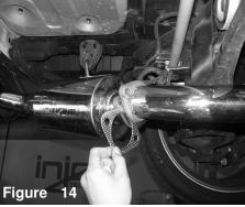
Install the flange and connect the two together.
