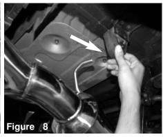
Attach the injen exhaust rear hanger to rubber hanger.
