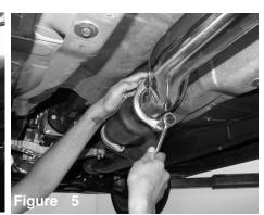
Tighten using factory nuts.
