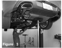
Remove the entire stock exhaust from the Catalytic
