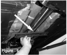
Loosen and remove the mid section bracket vehicle.
