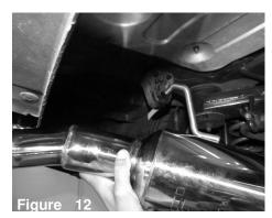
Install the driver side rear section and position he injen exhaust rear hanger to rubber hanger.
