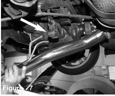
Install the passenger side rear section and position to rubber hangers and resonator.
