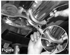
Install the 60mm gasket between the two parts and secure. Secure the two parts using provided M10 bolts and nuts. *DO NOT TIGHTEN!*
