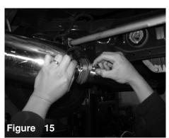
Secure the two parts using provided M10 bolts and nuts. *DO NOT TIGHTEN!*
