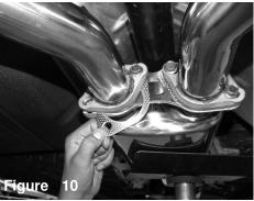
Install the 60mm gasket between the two parts and secure. Continue to install other side and position. **DO NOT TIGHTEN!**
