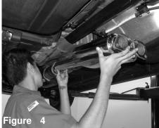
Install the midsection with resonator and secure.
