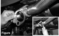
Place one supplied 60mm gasket and two M10 nuts and bolts connecting the right side muffler section flange to the mid-pipe flange. Use a 14mm rachet and socket to snug the two M14 nuts and bolts for now. Do not tighten them. Repeat this process for the left side muffler section.
