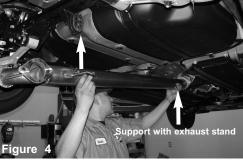
Position the Injen Mid-Y pipe into postion. Place the mid hanger onto the grommet. Make sure you support the front of the exhaust pipe with a exhaust stand.
