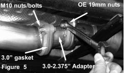
Place the supplied 3.0"-2.375" adapter in between the down pipe and injen exhaust pipe. Place a 3.0" gasket inbetween the Injen pipes. Use the OE 19mm nut on the down pipe and two M10 nuts and bolts on the Injen side to secure them together. This adapter will allow you to upgrade to the Optional Injen 3.0" down pipe.
