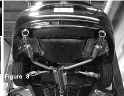
Make sure nothing comes into contact with any component and then make your final adjustments to the entire exhaust system. Use a 14mm socket and rachet secure all the
