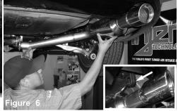
Once the mid-pipe is in place. Position the right side muffler section into the right side bumper cavity and then hang the muffler on the grommet.
