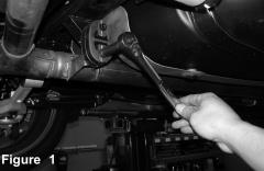
Use a 12mm socket and rachet to remove the 12mm bolt on the center hanger located near the stock exhaust "Y"
