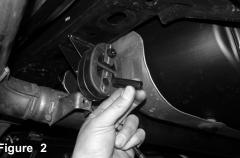
Pull the spacer out of the exhaust grommet from figure 1
