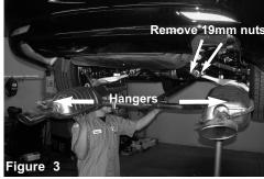
Remove the two 19mm nuts in front of the exhaust. Then detach the rear mufflers from the rear hangers and drop entire exhaust system from the vehicle.
