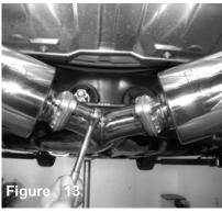
with nuts to secure the flanges together on both drivers side and passenger side.
