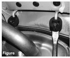
Pull back the rear isolators from the mufflers.
