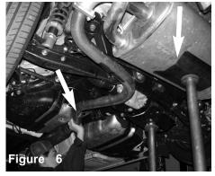
Using a support or extra person, remove the exhaust system from the vehicle.
