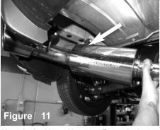
Now take the drivers side rear muffler section hanger and insert it into the rear exhaust grommet. Note: Flanges can rotate slightly for more adjustment.
