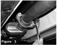
Loosen the 2 bolts holding in the exhaust system at the catalytic converter. Save the bolts to be used again in new exhaust system.
