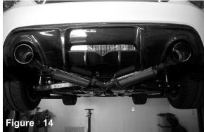
After the gasket is in place. Insert two M10 bolts Rear muffler section secured to Y-pipe sections. Make your final adjustment and make sure you have clearance with no iterference with the bumper or chassis components. you may now Tighten all the bolts supplied once all adjustment have been made and then recheck again.
