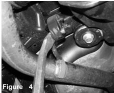
Pull back the rubber isolators from the exhaust system.
