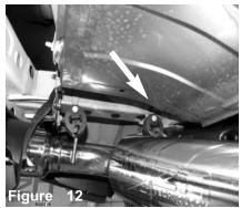
Place one 60mm gasket between the flange of the mid-pipe section and rear muffler section. Make sure that the haners are in the isolators.
