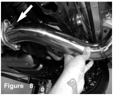
Install the Y-pipe using provided bolts and nuts. Secure the flanges using provided gasket. DO NOT TIGHTEN.
