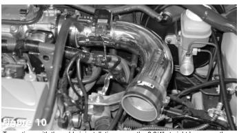
To continue with the cold air installation, press the 2 3/4" straight hose over the end of the primary intake, use two clamps on the hose but only tighten the clamp on the intake at this point.
