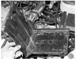
Remove the plastic battery tray before installing the cold air intake. This will allow more room through out the length of the secondary intake.
