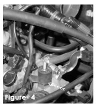
Screw the vibra-mount in place until it bottoms out.
