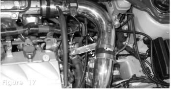
Now the top end of the secondary intake is pressed into the 2 3/4" hose located on the primary intake. Line up the intake for best possible fit before tightening any nuts, bolts or clamps.
