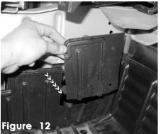
Take a razor and cut a 5" x 5" square opening below the frame leading into the bumper area.
