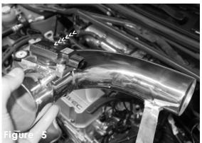
Remove the air temperature sensor from the stock air intake box. Insert the sensor into the machined adapter located on the air intake tube.
