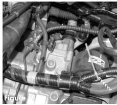
Place a zip tie around the harness to make sure it is safely tucked away from any moving objects.
