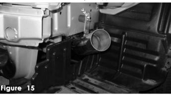
Line up the bracket on the secondary intake to the vibra-mount stud. Use the m6 flange nut and fender washer to secure the intake in place.
