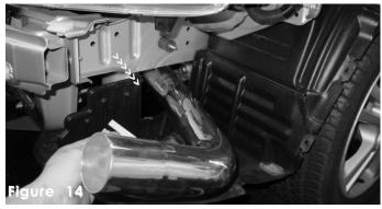
Inserts the secondary intake into the plastic opening and up into the engine compartment.
