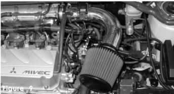
On rainy day always place the filter over the end of the primary intake. This system can be converted into a short ram.
