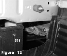
Screw the secondary vibra-mount into the pre-tapped hole on the wall of the frame of the car (A). The plastic guard has been cut and prepped for the installation of the secondary intake (B).
