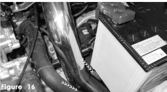
Allow plenty of clearance when installing the secondary intake. There should be clearance between the battery and the radiator hose.
