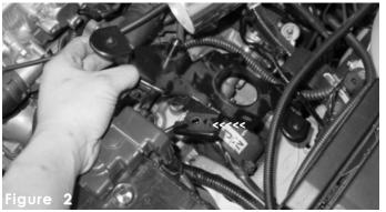
Remove all air intake ducting and air intake box leading to the throttle body. For this application it will be necessary to remove the black air intake brace to make room for the bracket on the intake.
