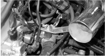
Line up the bracket on the intake to the vibra-mount stud and use an m6 flange nut and fender washer to hold it in place.
