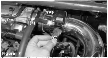
Press the top end of the primary intake into the straight hose on the throttle body and semi-tighten the clamp (A). Press the stock vacuum line over the 3/8" port on the intake (B). Plug the harness clip back on to the sensor until you hear a sharp snap (C)
