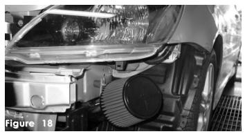
Press the filter on the end of the end of the secondary intake and tighten the clamp located on the filter neck.
