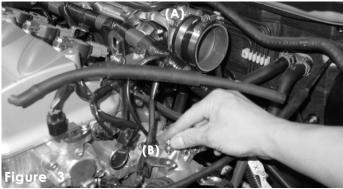
Press the 2 3/4" hose over the throttle body and use two clamps, tighten the clamp on the throttle body (A).Remove the zinc plated bolt from the brace(B) this is where the intake vibra-mount will be located.
