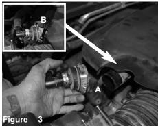
A) Loosen clamp on the crankcase coupler part of the airbox. B) Disconnect the crankcase coupler line from the air box.
