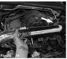
A) Install the intake tube into the vehicle and position the bracket to the vibramount and tube to the step hose
