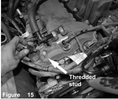
Locate the thredded stud on engine. With provided M6 vibramount, secure to the engine.
