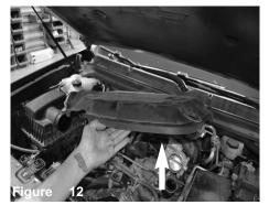
A) Remove the oil cap. B) Now lift up and remove the engine cover from the vehicle.
