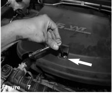
On the front of the engine cover next to the fitting, loosen the 2nd screw holding in the engine cover using 10mm socket or wrench.
