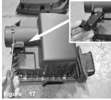
Loosen the 2 screws holding in the MAF sensor using T25 torx bit, and remove sensor from vehicle.
