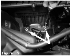
Loosen and remove the 2 nuts holding in the bottom air box using 10mm socket and ratchet.
