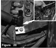
Now secure the bracket using provided nut and fender washer. Secure and tighten using 10mm wrench.
