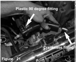
Remove factory coupler of the plastic 90 degree fitting. With provided 15mm attach the hose to the plastic 90 degree fitting and fitting on intake tube.
