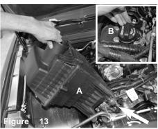
A) Now lift up and remove the airbox. B) Now install the oil cap to the engine.
