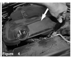
Loosen the clamp on the throttle body using 8mm nut driver.
