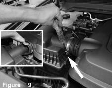
Loosen the clamp on the air box using 8mm nut driver. Remove the oil cap.
