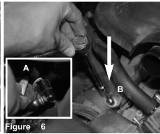
A) Disconnect the vacuum line in front of air box. B) Loosen the 10mm bolt on side of the engine cover.
