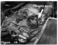
With clamps provided, attach the step hose to the throttle body. Tighten the clamp on the throttle body only using 8mm nut driver.
