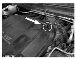
With 10mm socket and ratchet, loosen the screw on the back of the engine cover and remove.
