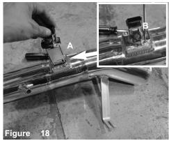
A) Now install the MAF sensor into the intake tube.
