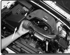
7. INow lift up and remove the air box assembly out of the vehicle.
