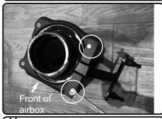
**11.** Install the provided Bracket to the powerflow box using provided M6 screws. Secure and tighten .
