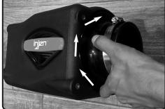
9. 1)Insert twist lock filter to the air box. 2)Once seated, rotate in either direction 1/4 turn till filter locks.
