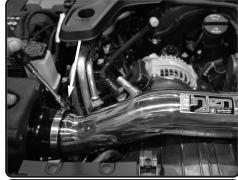
**19.** Tighten the clamp on the filter using 8mm nut driver.
