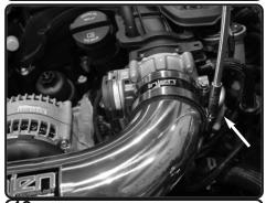
**18.** Position the intake for best fit. Tighte clamp 8mm nut driver.
