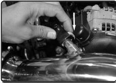
**21.** Re-connect the crank line to the intake tube fitting. MAke sure you hear the click.
