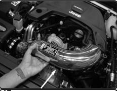
**17.** Install the intake tube to the vehicle. Postion to the hose and filter.
