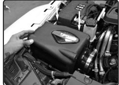
**14.** Powerflow box installed and seated properly.
