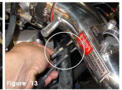
Take the two 4mm vacuum lines above the fuel rail and press them into the two small 3/16 vacuum ports on the intake.
