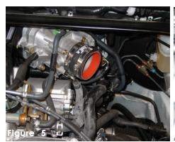
Place the 2 3/4 straight hose over the throttle body and use two clamps. Tighten the clamp on the throttle body side at this point.
