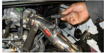
Remove the stock mass air flow sensor from the air intake box and press it into the machined adapter on the intake. Be sure not to break or pinch the O-ring along the base of the mass air flow sensor.
