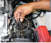
Take the 6mm vibra-mount and screw it into the stock air box bracket. Make sure it is fully screwed into the pre-tapped hole.
