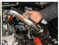
Take the assembled filter and intake and press the top end into the hose on the throttle body.
