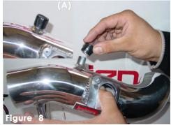
All 3.3L motors will require the 5/8 vacuum cap. Place the vacuum cap over the short 5/8 port on the intake. (See fig. A)
