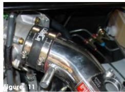
Once the intake has been adjusted continue to semitighten the clamp on the hose.
