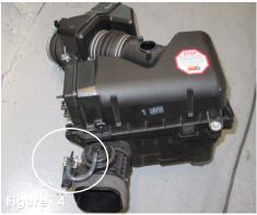
Note, the vacuum switching valve is intact with the air intake box which is no longer used.
