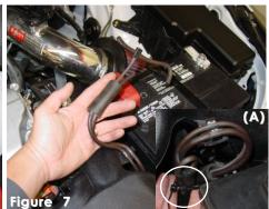
Take the wires that where connected to the vacuum switching valve and wire tie them away in a safe place. (See fig. A) The flapper valve has been illiminated so these wires can be tucked away in a safe place.
