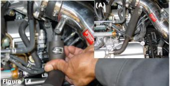
Take the stock breather hose at the crankcase and press the open end over the large port on the intake. (See fig. A)
