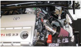
Top view of the air intake fully installed. Be sure to tighten all nuts, bolts, and clamps once the intake has been carefully aligned. Check the intake and vacuum lines for any rattling and/or vacuum leaks before moving forward with the test drive.
