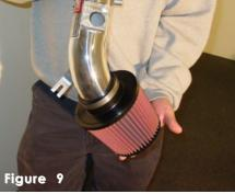
Press the filter on the end of the intake and tighten the clamp on the filter neck.
