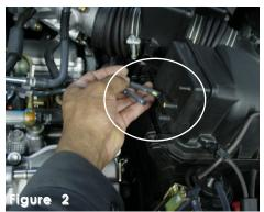
Remove the two 4mm lines connected to the solenoid Remove the entire stock air intake box from the vacuum switching valve controlling the air intake flap.
