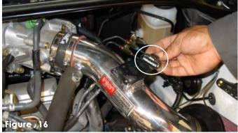
Use the stock self-tapping screws and secure the mass air flow sensor to the machined adapter.
