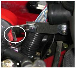
When the filter is pressed over the end of the composite adapter the L-bracket on the end of the 2020 bracket is slipped under the clamp located on the filter neck.
