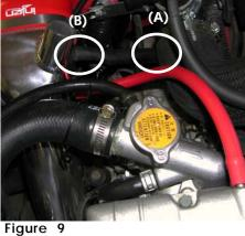
The stock 10mm vacuum line connected at the exhaust port (A) is pressed over the 1/2" port on the intake (B).
