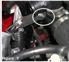
Attach the assembled 2020 and L-bracket to the vibramount stud. Use the m6 flange nut and fender washer (A) to hold the assembled brackets in place. The m8 flange nut and bolt are joining both brackets (B).
