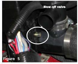
Remove the stock m6 bolt holding the fuse box in place. Screw the vibra-mount in place of the m6 bolt until it bottoms out.
