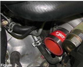
Press the 2 1/4" straight hose over the end of the turbo inlet and use the two small clamps.
