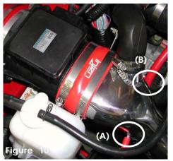
Replace the stock 4mm line that connects to the boost control solenoid and the 3/16 port on the intake (A). Do the same with the 8mm breather hose connected to the valve cover port and 3/8" port on the intake (B).
