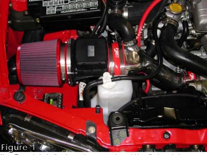
Note: The stock plastic elbow is reused to reconnect the stock blow-off valve to the large open port on the intake.
