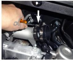
**10.** Place the 2.75"-3.00" step hose onto the turbo inlet. Only secure the clamp on turbo inlet for now.
