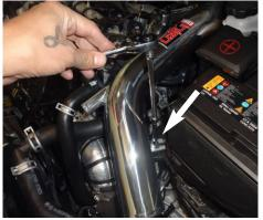
**13.** Secure the intake bracket to the vibra mount using the provide M6 nut and washer.
