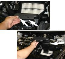
8. *Figure A:* Remove the two plastic clips from the front air intake duct. *Figure B:* Lift up and remove the front air intake duct.
