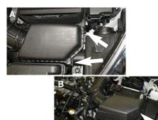
Figure A: Unclip the two tabs from the lower air box assembly to the upper air box assembly. <u>Figure B:</u> Detach the upper air box assembly from the lower assembly.
