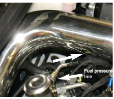
15. <u>CAUTION</u>: Make sure the bottom of the intake pipe does not rub on the high pressure fuel line. This line is connected to the fuel pressure regulator indicated in the photo.
