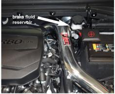
16. <u>CAUTION</u>: Make sure the intake pipe has adequate clearance from the brake fluid reservoir. Adjust the intake pipe for best possible fitment and then secure the all the clamps.
