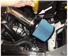
**17.** If installing the cold air intake, proceed to step 19. Place the filter onto the end of the intake pipe and then secure the clamp on the filter.
