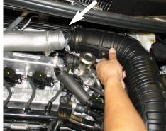
**5.** Loosen the clamp on the that is securing the intake tube to the turbo inlet. Detach the intake tube from the turbo inlet.
