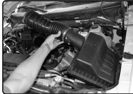
**2.** Disconnect the MAF sensor harness and unclip the 3 metal tabs holding the upper air box to the lower air box. Loosen the clamp on the air duct and then remove the upper box assembly and air filter panel.
