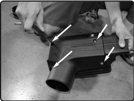
**6.** Use 4-M6X30 screws to secure the plenum to the Injen upper air box.
