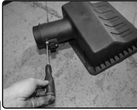
**3.** Use a torx screw driver to remove the screws to remove the MAF sensor from the stock OE air box assembly.
