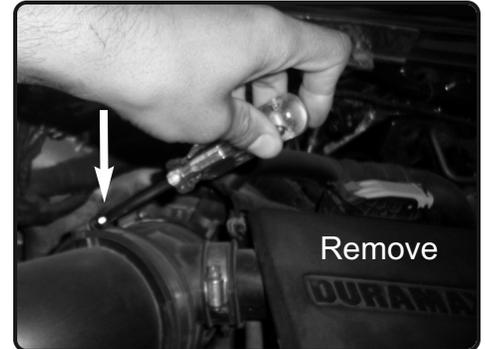
3. Loosen clamp on intake tube. Loosen the nut holding in the Duramax resonator box and remove. Lift up and remove the OEM air box out of vehicle.
