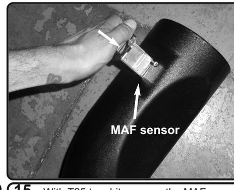
**15.** With T25 torx bit, remove the MAF sensor from the factory intake tube and install into new injen intake tube and secure using provided M4 screws.
