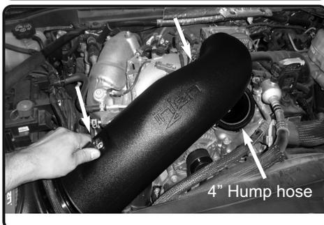
**16.** Install the provided 4" hump hose with clamps. Install the intake tube. *(coolant line is optional to run on top or below intake tube)* Position intake tube.
