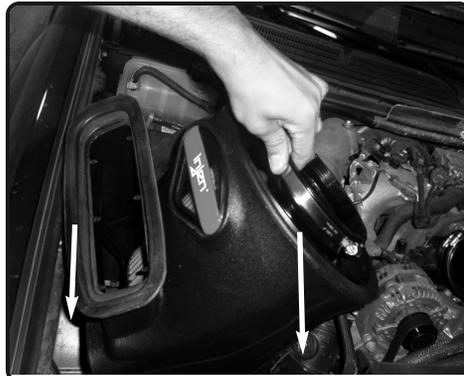
**13.** Install the injen airbox into the vehicle and position to the OEM air box location and secure.
