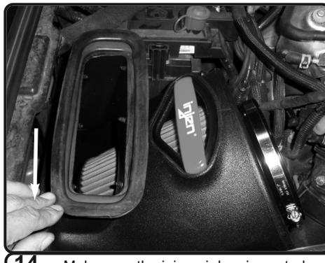
**14.** Make sure the injen air box is seated and secured properly into the OEM bracket. Make sure grommet from step 9 is locked in and seated in bracket.
