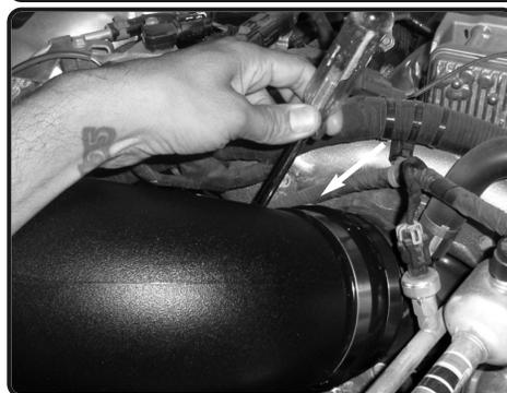
**18.** Secure and tighten the clamps on turbo using 8mm nut driver.
