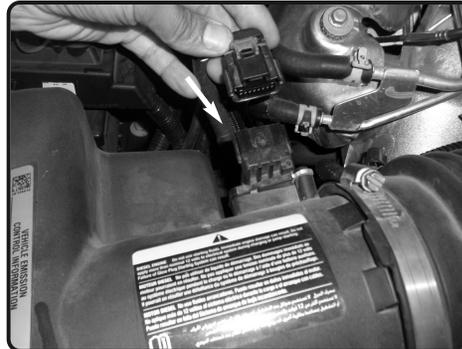
7. Disconnect the MAF sensor harness. Pull line away from the air box.
