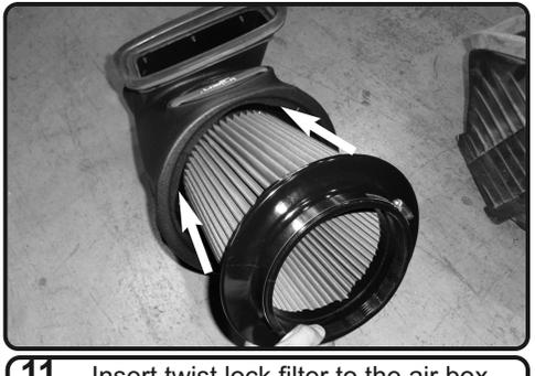
11. Insert twist lock filter to the air box
