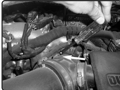
2. Loosen the clamp on turbo suing 8mm nut driver.
