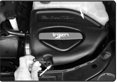
**10.** Install the air box assembly into the vehicle. Secure using OEM screw. Make sure the nipple fitting on back side of injen airbox is seated in the OEM grommet on fender well.
