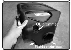
**9.** Remove the factory rubber grommet with washer from OEM airbox and install to the new injen airbox. Attach the Rubber trim to the bottom of the air box.
