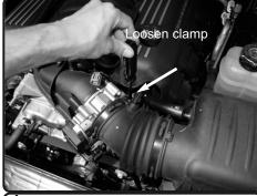
**4.** Loosen the clamp on throttle body using 8mm nut driver.
