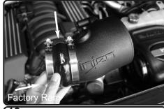
**12.** Install the provided 3.5" hump hose with clamps to the intake tube.
