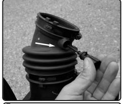
**7.** Now carefully remove the temperature sensor from the intake tube.
