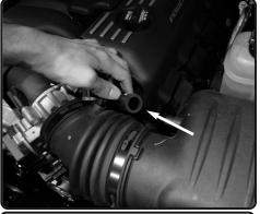
**3.** Pull back crank case line from airbox fitting.
