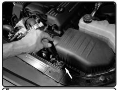
**5.** Loosen the bolt holding in the airbox using 8mm nut driver.
