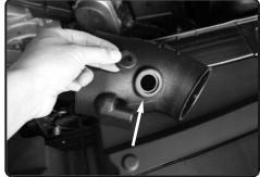
**11.** Install the provided grommet to the hole on the intake tube.
