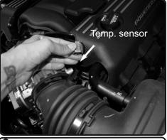
**2.** Disconnect the Temperature sensor harness.
