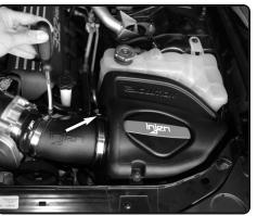
**14.** Adjust for fitment and tighten all clamps using 8mm nut driver.
