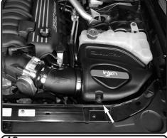
**18.** Secure and tighten the air box screw from step 10
