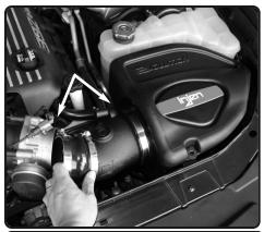
**13.** Install the intake tube to the filter and the hose to the throttle body.
