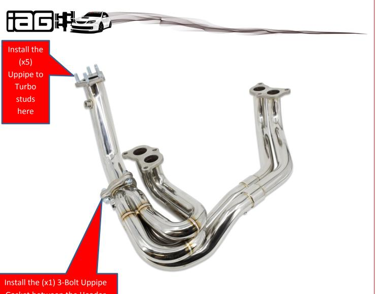
Gasket between the Header and Uppipe using the supplied (x3) Nuts & Bolts
