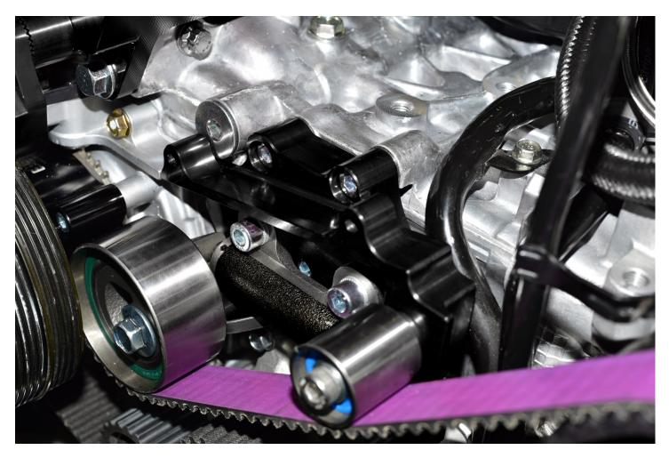
This picture shows the correct mounting and timing belt routing.
