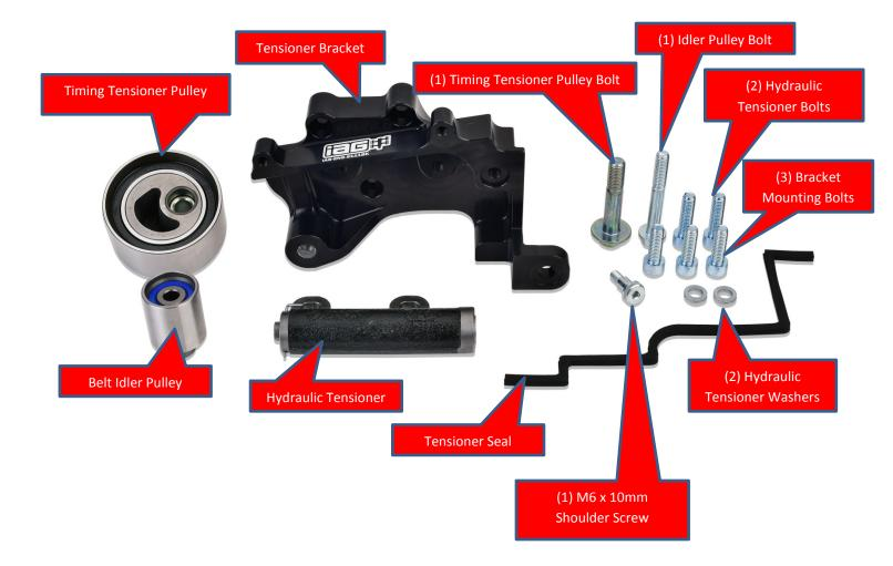
1. Apply included foam seal to the back side of the large tensioner bracket. This seal goes between the block and the tensioner bracket.
