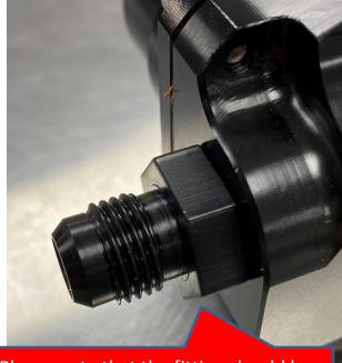
Please note that the fitting should be fully flush when installed properly. Torque these fittings to 16 ft/lbs.
