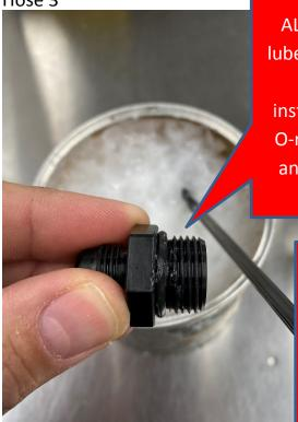
**ALWAYS** apply lube to all O-rings for this installation. Dry O-rings can tear and that's bad.
