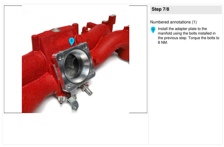
IAG-AFD-2027 - IAG Big Bore 76mm Throttle Body & Adapter Package for OEM & Cosworth Manifolds rev. | 46804 v3 [Published] 2022-09-08 12:08 UTC
