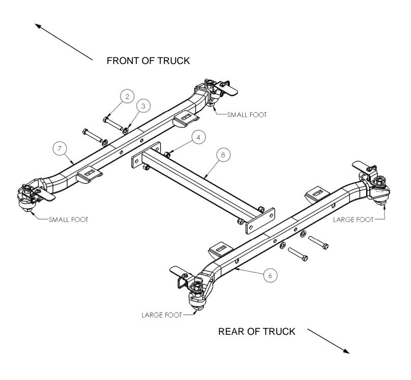
4. Place the assembled Ram 5<sup>th</sup> Wheel adaptor in your truck bed. The handles and T-bolts must be rotated into the Un-locked position.
