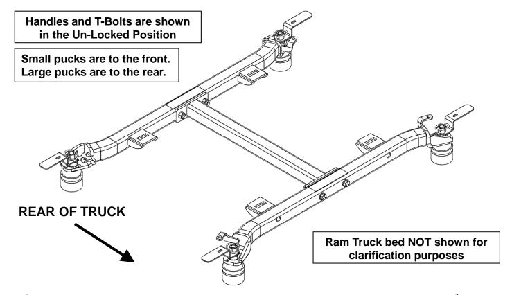
6. Once the Ram adaptor is installed; make sure the Adaptor Rails sit FLAT with the Ram 5<sup>th</sup> Wheel "pucks" at ALL 4 contact locations.
