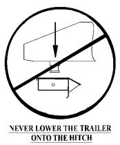
NEVER LOWER THE KING PIN INTO THE HITCH USING THE TRAILER JACKS. THIS IS A VERY DANGEROUS PRACTICE AND WILL RESULT IN THE KING PIN SITTING ON TOP OF HITCH INSTEAD OF INSIDE. THE TRAILER COULD THEN BECOME DETACHED FROM THE TRUCK DURING TOWING CAUSING SERIOUS DAMAGE AND POSSIBLY INJURY OR DEATH.
