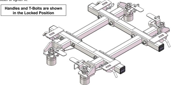
4. Once the Adaptor is installed; make sure the Adaptor Rails (#2) sit **FLAT** with the Ford 5<sup>th</sup> Wheel "pucks" at **ALL** 4 contact locations.
