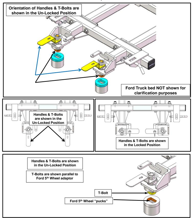
3. Once the Adaptor is installed; turn handles into the locked position. This may require adjusting the T-bolts for a looser or tighter fit.
