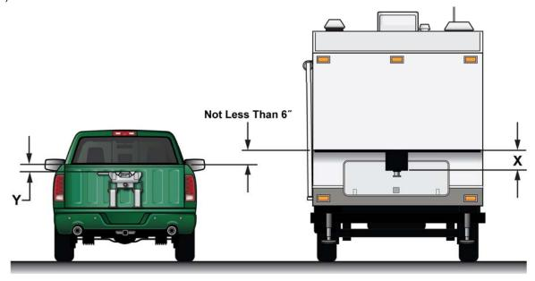
2. With top face of head level measure up to top of pickup box (dimension Y in Figure 1). On the trailer measure up from the face of the pin box to the underneath of the trailer (dimension X in Figure 1). Measurement X less measurement Y gives the amount of clearance between the top of the pickup box and the underneath of the trailer.
