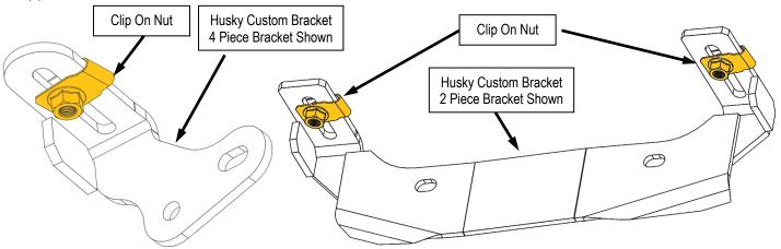
2: Install the 5/8"-11 hex head bolts & 5/8" hardware provided in the Husky Custom Bracket kit. DO NOT USE with a carriage bolt; you will NOT be able to tighten the bolt.
