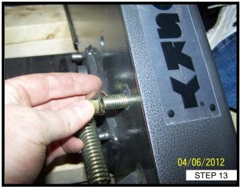
Insert the (5) new ½ hex bolts from the outside of the housing and thread the lock nuts on.
