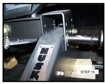
Tighten lock nuts to 75 lbs.-ft. Also tighten the (2) cross member nuts you loosened earlier to 75 lbs.-ft.
