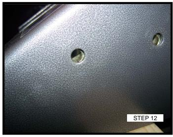
Slide upper rail in until the bushings line up with the housing holes.
