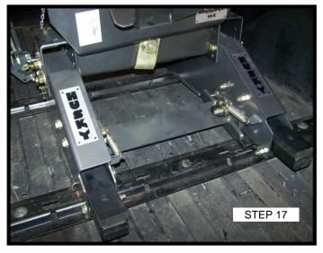
Remove 2 x 4 blocks and guide base rail tabs back into the base rail slots and insert the (4) base rail pins and clips. Check system for free sliding forward and backwards and adjust if necessary.
