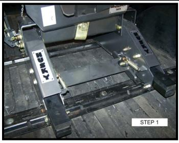
Remove base rail pins and clips.
