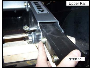
Carefully guide upper rail assembly with plastic facing down as shown.
