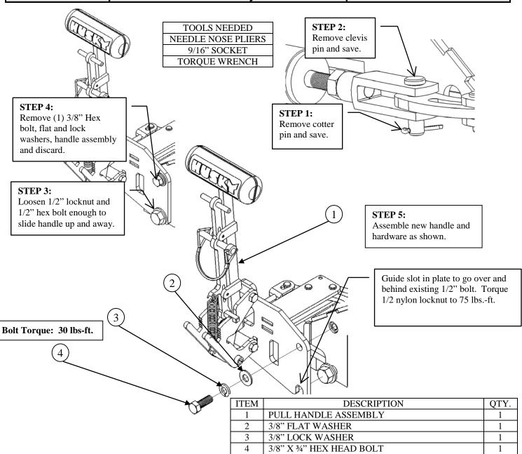
**IMPORTANT!** Check the operation of the flipper plates after new handle is assembled to ensure proper contact with the stop tabs is made. Make adjustments per the 16K Husky-10 instructions if necessary.
