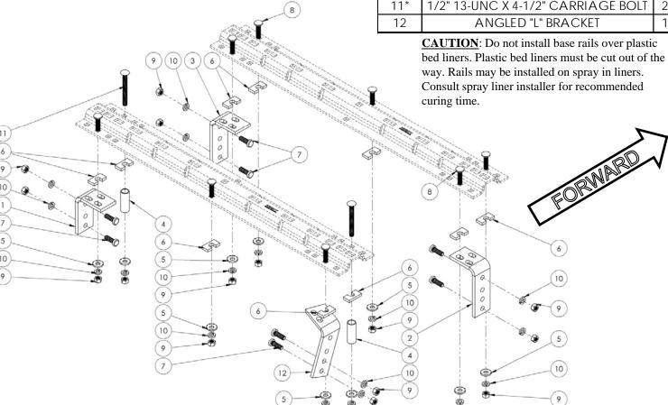
This adapter kit is to be used with install kit 31622 "Fit #10". This means omitting the passenger side rear bracket and installing a bushing and carriage head bolt the same as on the driver side rear is. Then install the bracket from this kit as shown below.
