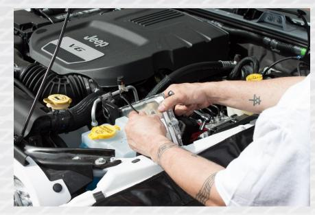
5. Reinstall the newly provided PCM in the bracket, taking note to reconnect the ground wire removed in step 3 along the way.
