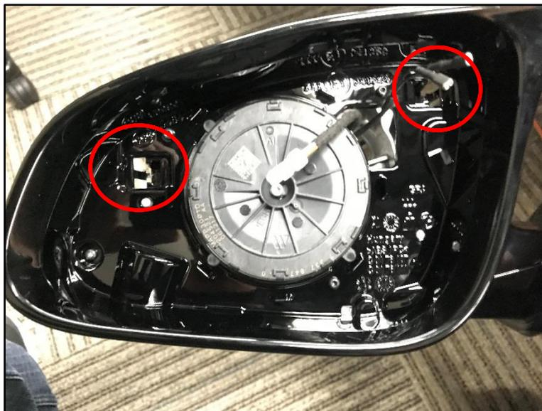
6. As you install the mirror cap, take care to align the tab on top before snapping it in to place. Once aligned, snap the mirror cap on. Check all the edges, to ensure it's installed securely.
