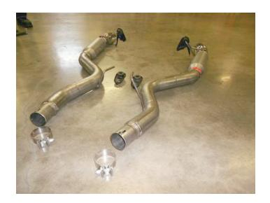
7. Remove nuts from stock and Flowmaster clamps, apply anti-seize compound to bolts and re-install nuts.
