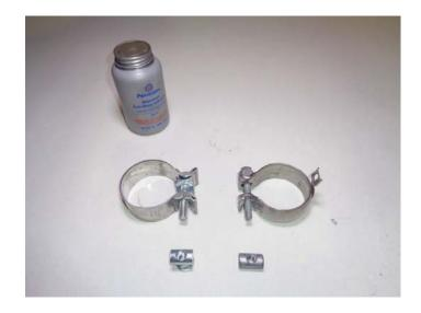
www.flowmastermufflers.com Technical Support (707) 544-4761 12. Place 2.5" band clamps (x2) (MC250BS) onto Scavenger assembly (26701S) inlets. Connect scavenger (with FM logo facing floor) to factory head pipes and slide it in approximately three inches. Tighten clamps just enough to allow for adjustment.
