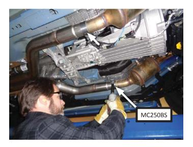
Place 3" band clamps (x2) (MC300BS) onto left mid pipe (26702S) and right mid pipe (26703S). Connect pipes to scavenger outlets as shown. Tighten clamps just enough to allow for adjustment.
