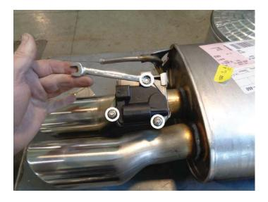
8. Lift actuator (with heatshield and spring attached) from factory valve assembly.
