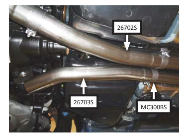
Place 3" band clamps (x2) (MC300BS) onto right muffler assembly (853063-509) and left muffler assembly (853063-510) inlets. Connect right muffler assembly completely to right mid pipe then reinstall front and rear mounts. Repeat with left muffler assembly on driver side of vehicle.
