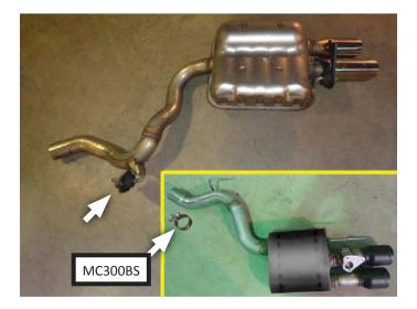
7. Remove nuts (x3) securing exhaust valve actuator to exhaust valve. Retain grounding clips aside for re-use.
