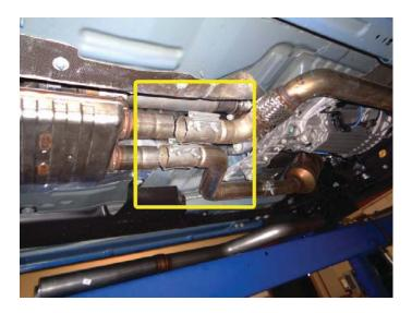
4. Unbolt mounts (just behind rear differential) and unplug valve actuators located at rear of factory mufflers. Slide exhaust system forward out of rear mounts and onto floor, while leaving front mounts attached. Then remove and retain rear mounts and factory mufflers.
