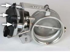
11. Remove nuts from stock and Flowmaster clamps, apply anti-seize compound to bolts and re-install nuts.
