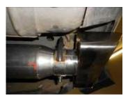
2) Place the left side stainless tip **#ST434** over the left muffler outlet, the 484HA clamp hanger with fit over the tip. Adjust the tip to the correct position and tighten the clamp enough to hold, but still allow for adjustment. Repeat this step with tip **#ST433** on the right side of the vehicle.
