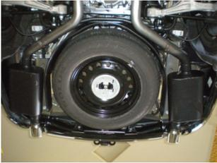
6) Place a provided clamp onto the inlet of muffler **#852562-255** and put up into position on the right outlet of the scavenger assembly. Slide the pipes fully together and connect the two hangers on the muffler assembly to the rubber mounts on the vehicle. Tighten the clamp at the inlet enough to hold, but still allow for adjustment. Repeat this step on the left side with muffler **#852562-254**.
