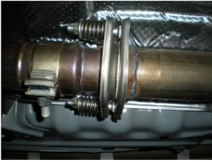
5) Take the provided M10-1.5x60mm bolts and slide on the flat washer. Then, put the bolts thru the flanges and slide on the provided steel spacer sleeves and the springs and nuts removed in step 2 above. Tighten down the fasteners until the nuts bottom out on the steel spacer sleeves.
