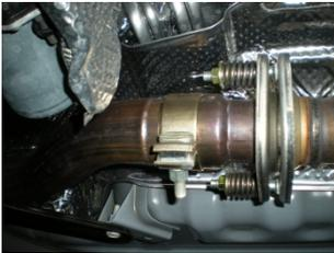
2) Begin by supporting the front and the rear of the system with a stand. Make your way forward from the rear and remove all of the wire hangers on the system from the rubber mounts on the vehicle. Then at the front flange connections, remove the nuts on the spring bolts and set the hardware aside, the springs and nuts will be reused with the Flowmaster system. With the help of an assistant, you can now lower the stands and remove the entire system from the vehicle and set aside.
