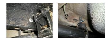
2) On the inside of the rear frame rails, roughly 10" forward of the bumper, you will find large holes that will be used to mount the tailpipe hanger brackets. You should see a round hole in the center of the frame rail. Place a supplied 3/8" x 3" bolt with a **#HA226** square backing plate installed through the hole from the outside of the frame to the inside. Place a **#HA572** hanger bracket onto the end of the bolt and secure with the nuts and lock washers provided.
