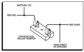
Figure 4 Wiring the Dual Ballast Resistor.
