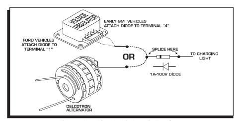
Figure 5 Installing the Diode to fix Run-On.
