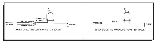
Figure 3 Connecting a Theft Deterrent Switch Through the MSD Ignition.
