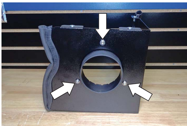
15. Assemble the air filter adapter (3) to the heat shield using M6 screws (13), lock washers (8) and flat washers (7).
