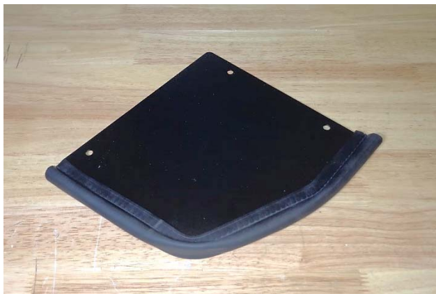
14. Attach gasket to the heat shield cover (5).
