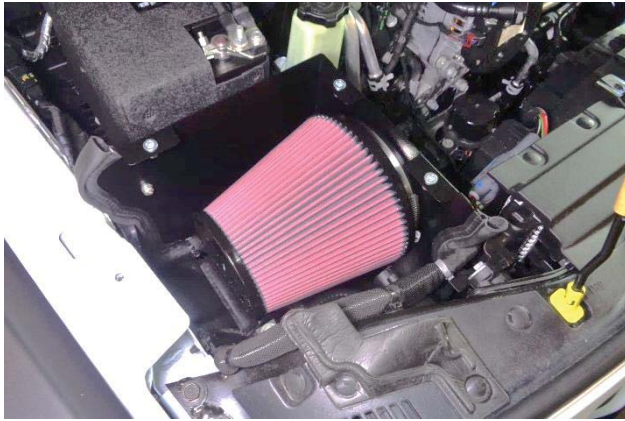
25. Place the #104 screw clamp (2) on the air filter (1), and the filter on the filter adapter, then tighten the clamp.
