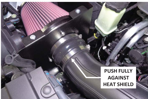
27. Push the reducing coupler fully up against the heat shield, then tighten the heat shield clamp.
