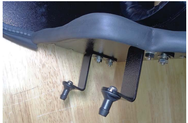
17. Fasten a barbed pin (14) to each bracket, using an M6 screw (13), lock washer (8) and flat washer (7).
