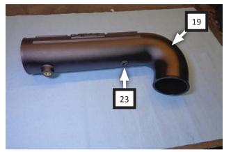
Insert grommet (23) into intake tube (19). Moistening grommet with soapy water will ease insertion.
