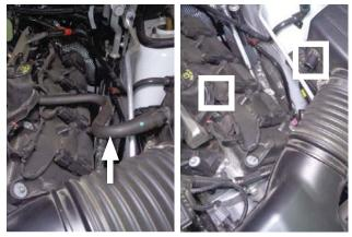
4. Disconnect PCV hose from oil fill and airbox then remove it from engine compartment.
