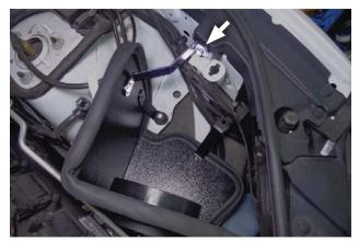
Install assembled heat shield into vehicle by pushing grommets (x2) onto pins. Re-install stock bolt (removed step 13) onto vehicle mount through bracket.
