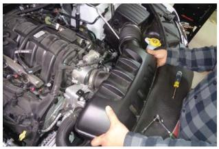
8. Remove resonator from engine compartment.
