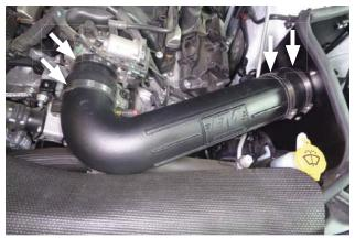
Push couplers flush against heat shield and throttle body before fastening outermost screw clamps (x2). Center intake tube between couplers then tighten remaining screw clamps (x2).
