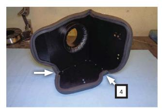
Starting at corner indicated, press heat shield gasket (4) gradually around edge of heat shield then trim to fit.
