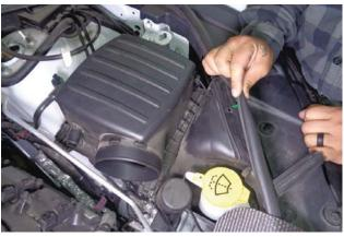
10. Unclip trim seal from corner of inlet duct.
