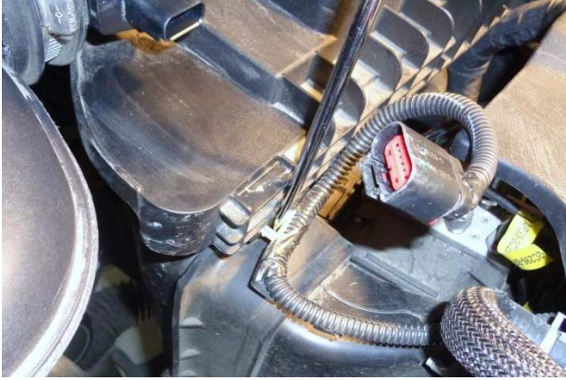
7. Use a flat-tip screwdriver to release the clip securing the MAF lead to the airbox.
