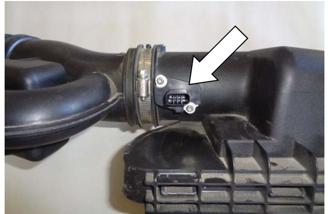
11. Remove the MAF sensor from the airbox, then remove the stock gasket from the sensor. CAUTION: The sensor is delicate! Handle it with care, and store it in a safe location until reinstallation.
