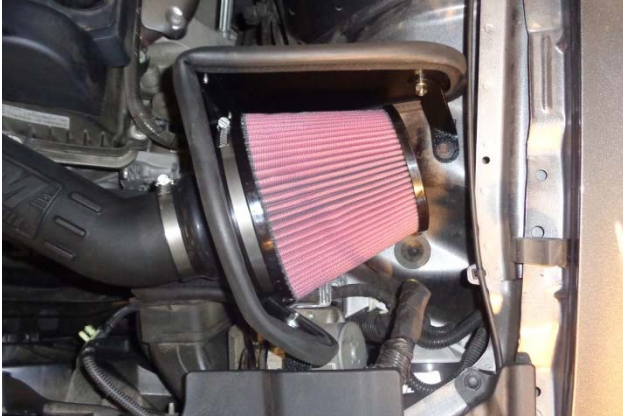
31. Install clamp (2) on air filter (1), then install filter on filter adapter and tighten clamp.
