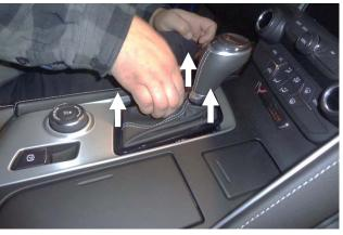
4. Carefully feel through the boot, and lift the bezel out of the center console.
