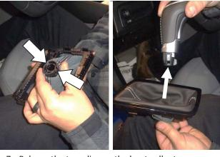
7. Release the two clips on the boot collar to disassemble the shift knob from the collar.
