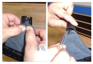
8. Carefully pull the collar off the inside of the shift boot. **NOTE: The parts are glued together. Work carefully to avoid tearing the boot.**
