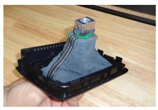
11. Use the cable tie to fasten the boot to the shifter handle at the boot groove, and trim off the excess cable tie. Back the set screws out so that they do not interfere with the shift lever in the next step.
