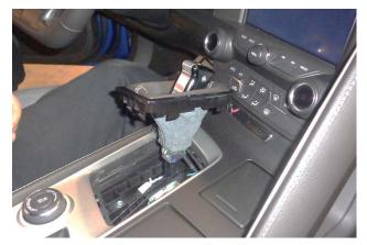
12. Slip the assembled handle and boot over the shift lever.
