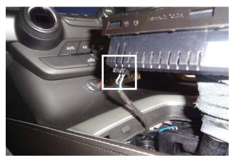
14. Connect the electrical plug to the bezel.
