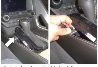
5. At the front driver side of the bezel, disconnect the electrical plug.
