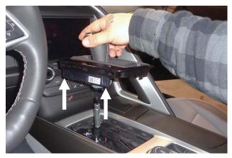
6. Remove the assembled shift knob and boot off of the shift lever.
