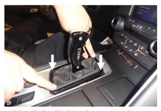
15. Snap the bezel back into the center console.
