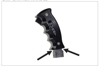
9. Install the set screws (2) in the base of the shifter handle (1). Turn the screws in until they are flush with the surface. Also, note the boot grooves on the front and rear of the handle.
