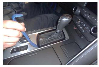
3. Use a trim removal tool to separate the shift boot bezel from the center console.
