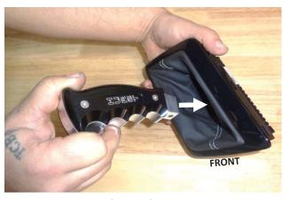
10. Insert the base of the shifter handle through the boot opening, with the finger grooves pointing toward the front of the boot.
