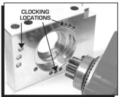
Figure 1 Clocking the Starter for Clearance.
