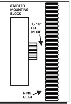
Figure 2 Checking Pinion Clearance.
