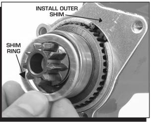
Figure 3 Installing the Pinion Shim Spacers.
