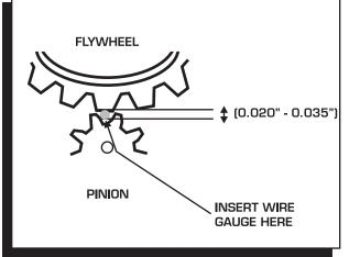
Figure 4 Checking Gear Mesh.
