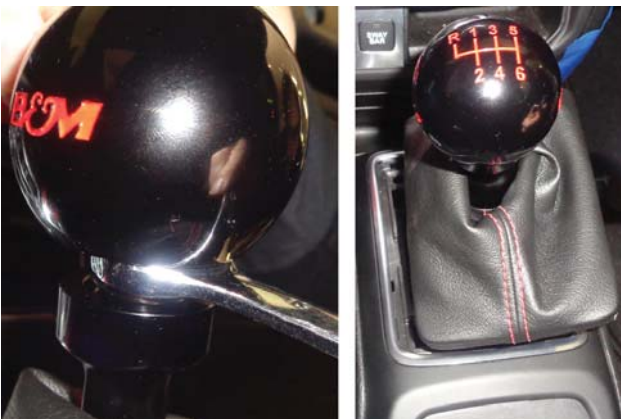
45. Turn knob back until it is aligned to your preference, then adjust jam nut to set knob in place.
