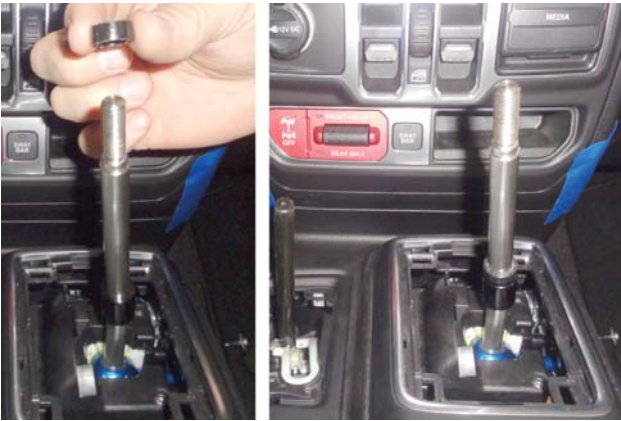
38. Install rubber stop (removed step 19) onto shifter assembly until it rests on lockout collar.
