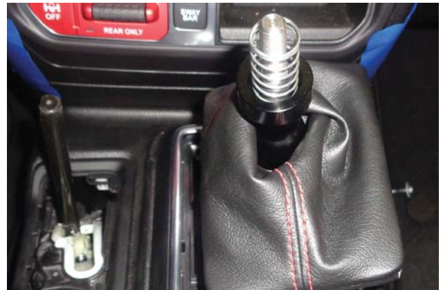
42. Place spring (removed step 5) onto shifter so it rests in reverse lockout.
