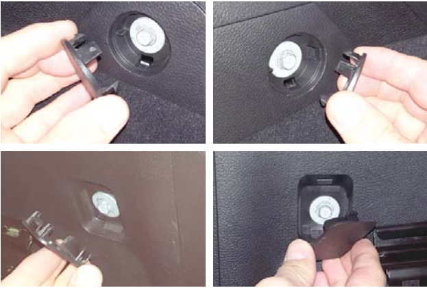
13. Remove (x4 ea.) plastic caps and screws from all four corners of console. Retain them for later use.
