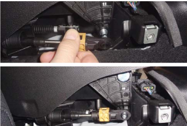
33. Install side cable onto side pivot arm, accessed from front passenger side of console.
