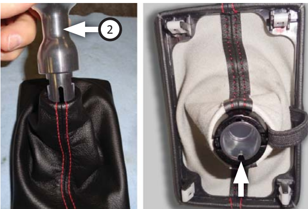
26. Align slot on reverse lockout (2) toward rear side of boot. Install reverse lockout into boot.
