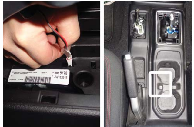
36. Plug cupholder wire back into console then replace console top.
