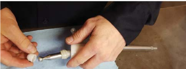
20. Remove cable pivot cup from shifter and retain it for later use.
