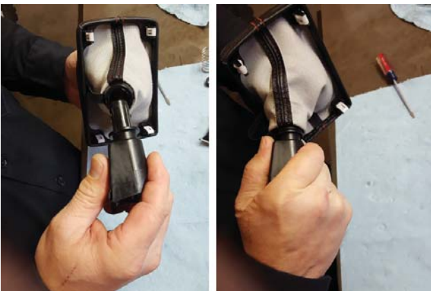
27. Insert reverse lockout factory bottom (removed step 24) into boot aligned with slot and press it into reverse lockout top until components click together.
