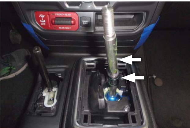
39. Apply grease to stem of shifter handle and collar.
