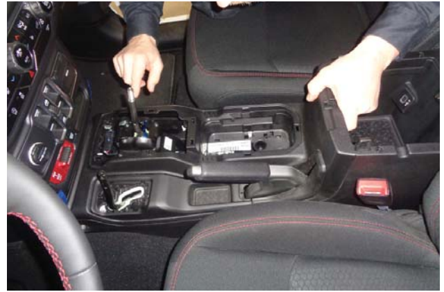
34. Replace console back in place as shown.
