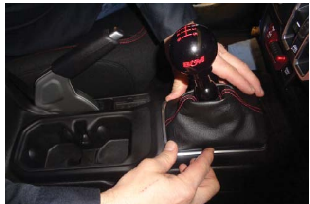
47. Set boot down into console in place.
