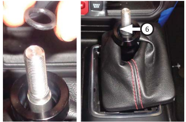
41. Install O-ring (6) onto shift stem so it rests in groove as shown.
