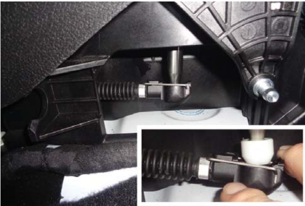
32. Install lower cable onto pivot cup, accessed from front passenger side of console.
