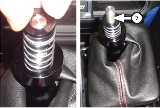
43. Thread jam nut (7) onto shifter stem then finger-tighten it fully.
