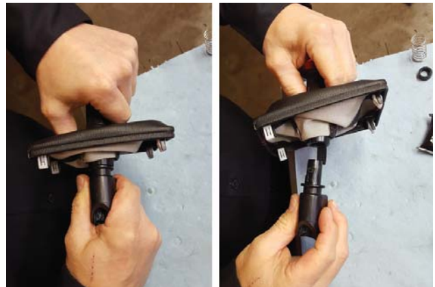
24. Pull factory reverse lockout bottom from stock shifter handle assembly (removed step 10) and retain it for later use.
