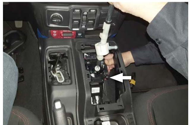
18. Lift shift lever upward while rotating side pivot arm upward to release shifter from base. Remove and retain shifter for later use.
