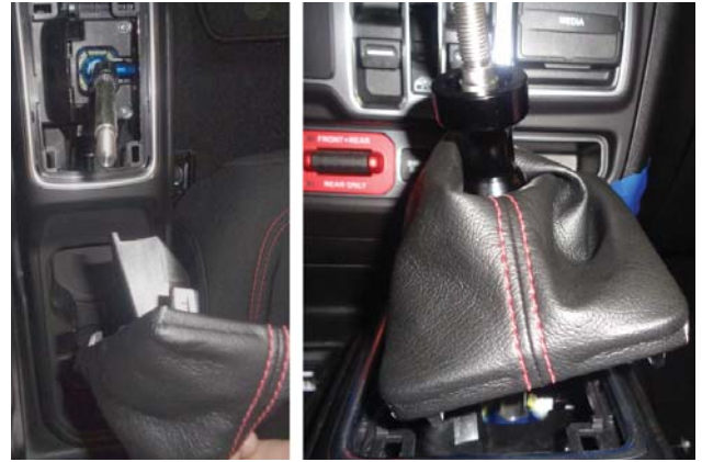
40. Install shifter lockout assembly onto shifter stem.
