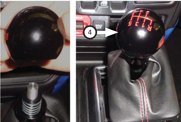
44. Install knob (4) onto shifter stem then finger-tighten it fully.
