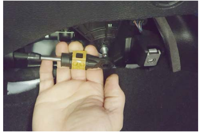
16. Disassemble side cable from side pivot arm, accessed on front passenger side of console.
