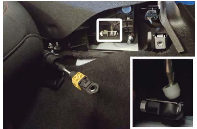
17. Disassemble lower cable from pivot cup, accessed on front passenger side of console.
