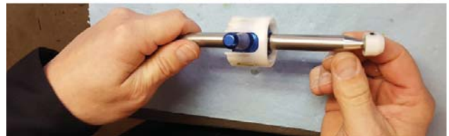
23. Apply grease from kit to pivot cup housing (removed step 21) and pivot on shifter assembly. Install pivot cup housing onto shifter assembly.
