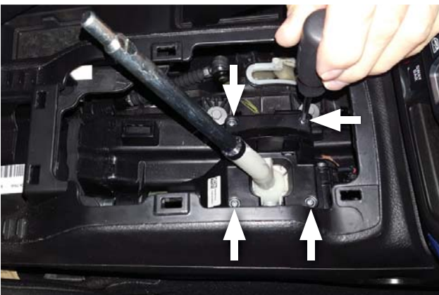
15. Remove screws (x4) and pivot cover plate from around base of shifter.
