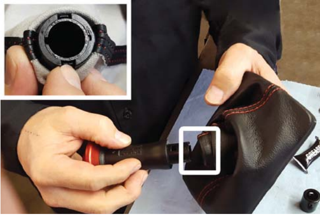
25. Remove factory reverse lockout top from boot by unclipping it at its base then pulling it out. Retain boot for next step.
