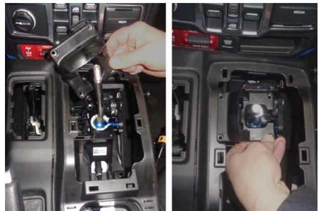
30. Set pivot cover plate (removed step 15) into position at base of shifter as shown.
