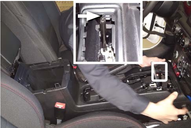
14. Pull up on front of console until you can use transfer case shifter stem as a prop for support.
