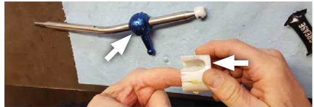
22. Apply grease from kit to pivot cup (removed step 20) and bottom pivot arm of shifter assembly (1) . Then install pivot cup onto shifter assembly.
