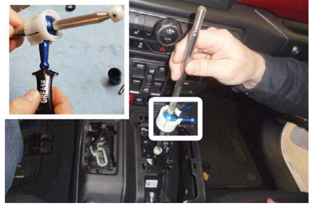
28. Apply grease to shifter side pivot arm. Set shifter assembly into position in vehicle where shown.
