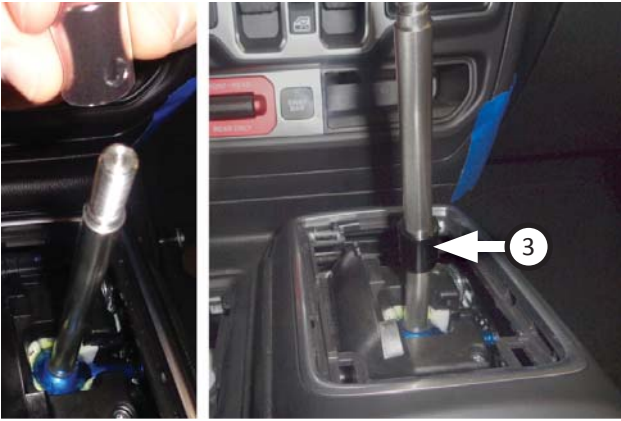
37. Slide lockout collar (3) back onto shifter assembly with large side hole oriented towards passenger seat.
