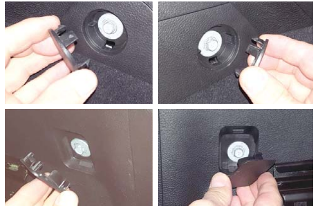
35. Install (x4 ea.) plastic caps and screws (removed step 13) into all four corners of console.
