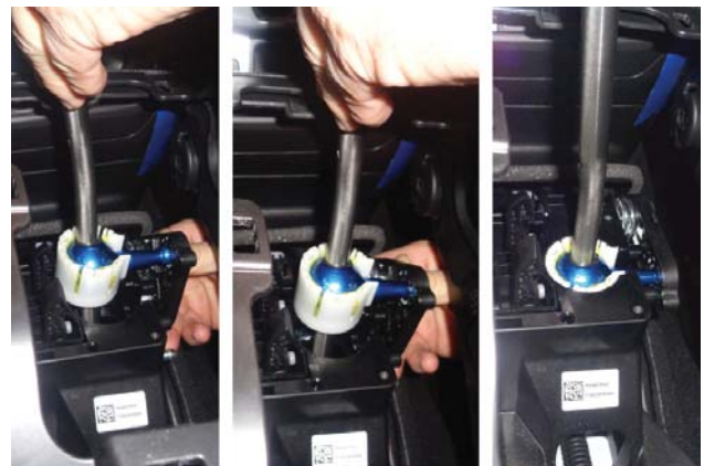
29. On shifter base, rotate side pivot arm upward, align shift lever over base and snap side pivot ball into pivot arm. Then push shift lever and main pivot ball cup into shifter base until they are flush at top.
