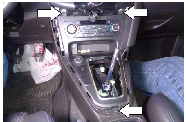
61. Install and tighten the 3 power panel screws.
