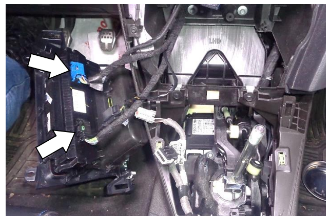
24. Disconnect the blue (AUTO) and black (AC) connectors, and remove the power panel from the vehicle.
