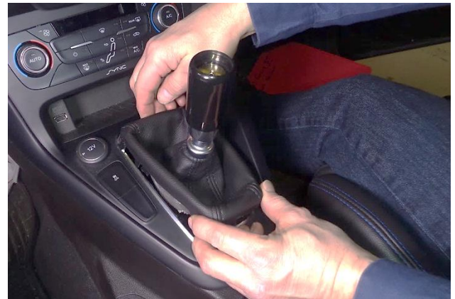
72. Snap the boot into the center console.
