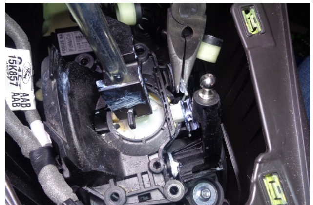
30. Use pliers to lift the top leg of the centering spring up off the rubber grommet on the side shaft.
