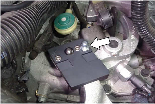
43. Apply medium strength thread-locking fluid to one of the ball studs (6) and install it in the shift plate.
