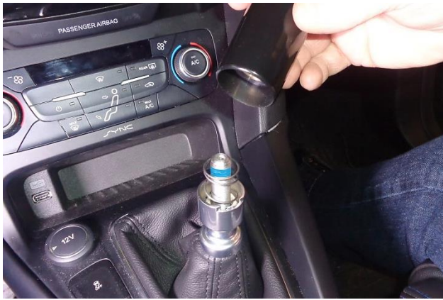
68. Apply medium strength thread-locking fluid to the first 4 or 5 threads on the shifter lever. CAUTION: Do not get thread-locking fluid on the reverse lockout return spring.
