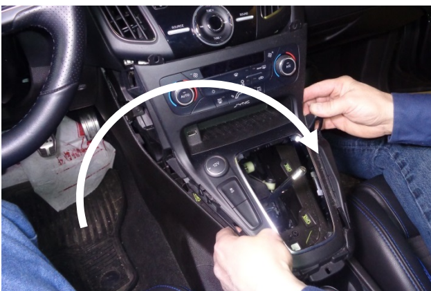
58. Carefully flip the power panel back over the center console.
