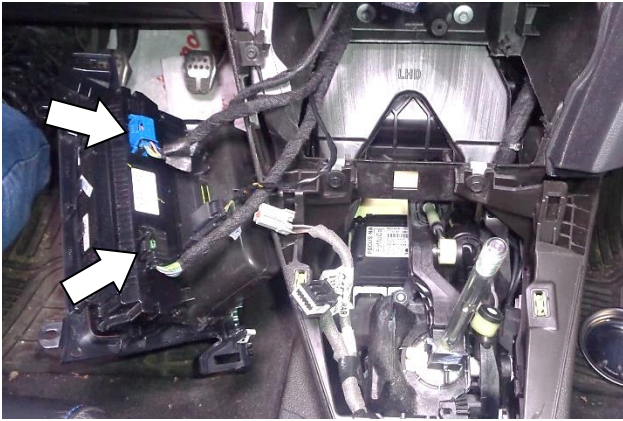
56. On 2015–2018 models, reconnect the blue (AUTO) and black (AC) connectors to the power panel, and continue with Step 57 below. • For 2013–2014 models, go to Step 65.
