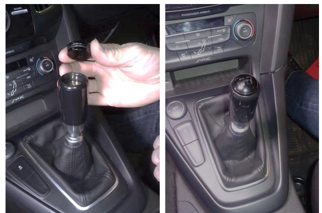
73. Lightly grease the O-ring (2) and install it on the cap (1). Then align the logo as desired and press the cap into the knob. Go to Step 77.
