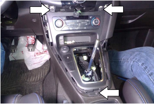
19. Remove the 3 power panel screws.
