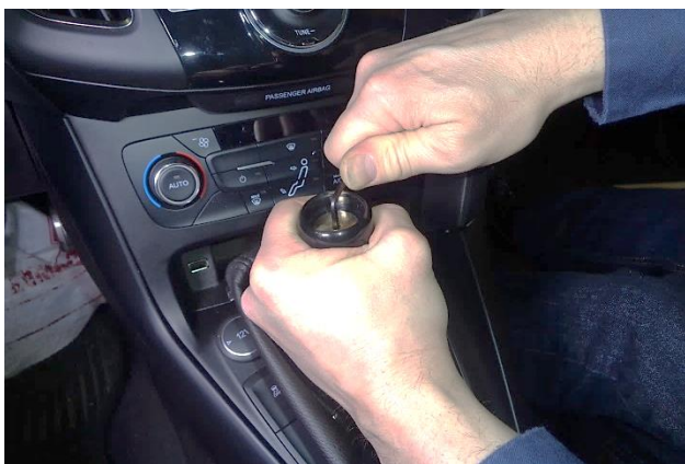
70. Firmly grasp the knob and tighten the set screw.
