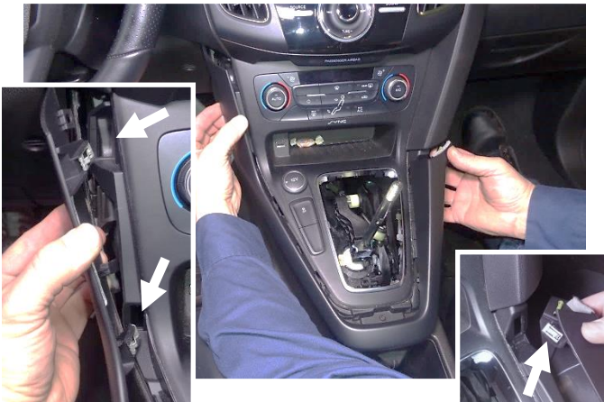
63. Reinstall the shift console trim, taking care to engage the 2 clips on the left, and the 1 clip on the right.
