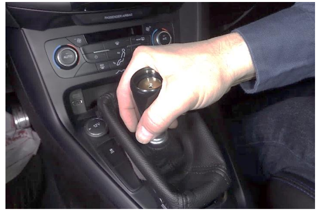
71. Move the shift lever into and out of REVERSE to verify correct operation of the reverse lockout. The reverse lockout lever should lift just high enough to clear the lockout notch on the shifter housing without touching. Adjust the height of the shift knob if required.
