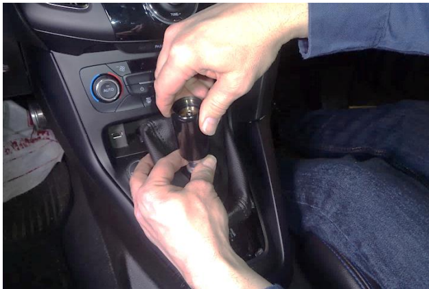
69. Thread the knob onto the lever. When it begins to drag against the reverse lockout collar, back it off approximately 1-1/2 turns.
