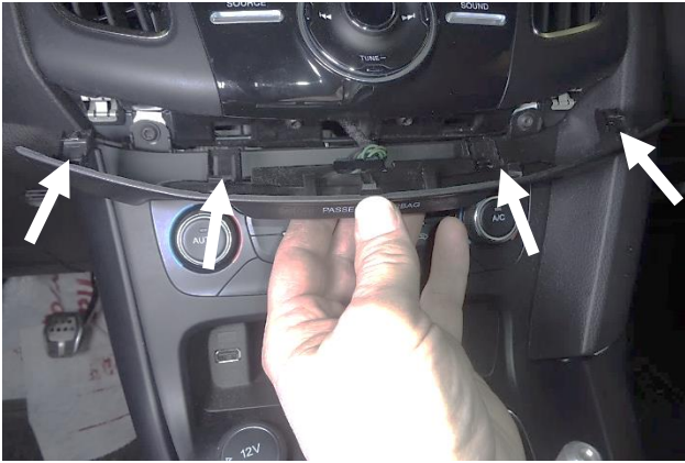
62. Reconnect the center panel bezel plug. Then line up the 4 clips on the bezel with their slots on the panel and reinstall the bezel.
