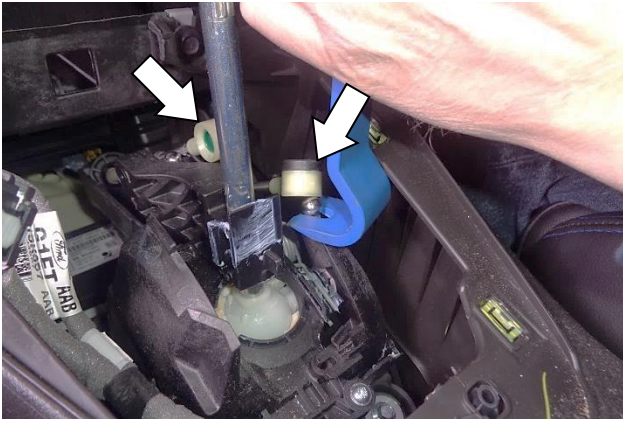
25. Carefully pry the 2 shifter cable ends off of their ball studs.
