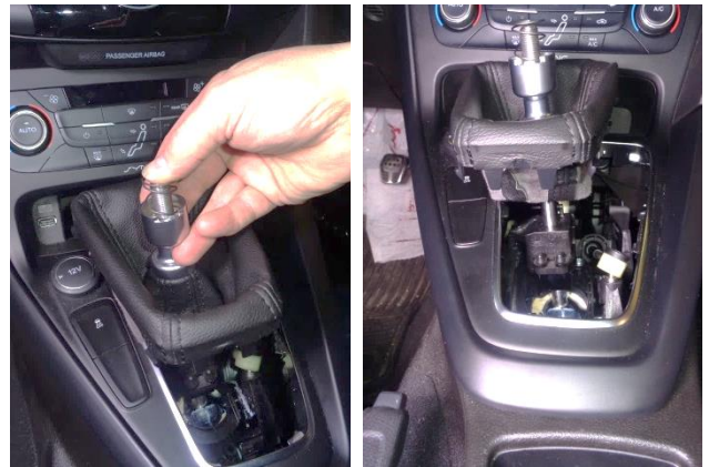
66. Move the shift lever into REVERSE gear.
