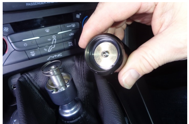
67. Install the set screw (3) in the shift knob (4), leaving 2-3 threads exposed.
