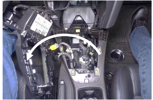
22. Carefully flip the panel toward the left, taking care not to strain the 4 electrical connectors.
