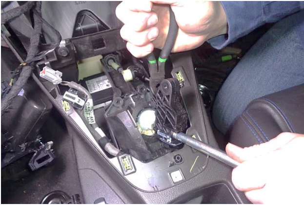
31. While holding the spring open, remove the shift lever and shifter top housing from the bottom housing.
