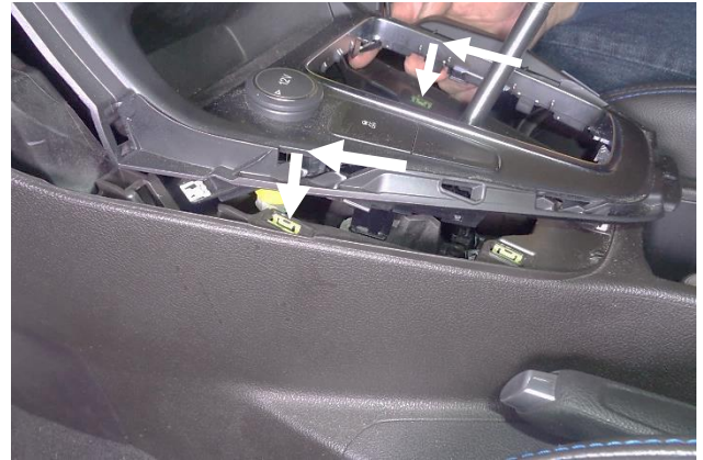
60. Install the power panel with a “forward-then-down” motion (the reverse of Steps 21 and 20). First move the panel forward, inserting its alignment tabs in their slots in the center dash. Then push it downward, snapping it into the 4 clips in the center console.
