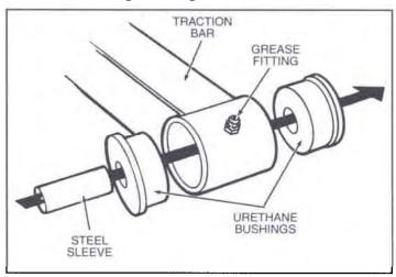
2. Apply lubricant (supplied) to polyurethane bushings and steel sleeves, then install into eyelet ends as shown.
