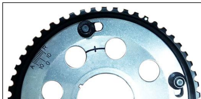
Figure 6: Indexing the Cam Hub for Drilling & Drilling the Cam Hub
