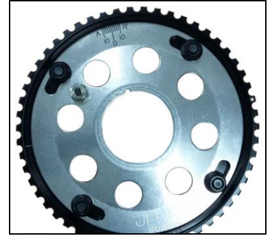
Figure 9: Finished Cam Hub
