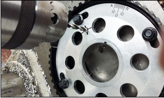
Figure 7: Drilling the Cam Hub
