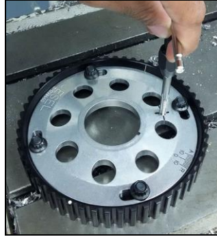
Figure 8: Tapping the Cam Hub
