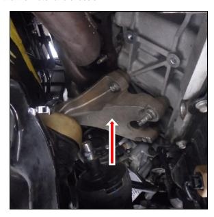
10. Repeat step 9 on the right side by removing (x2) 13mm head bolts, (x2) 13mm head nuts and (x1) 15mm head nut supporting the right side engine mount to the motor and chassis.
