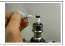
Screw knob onto handle until the bottom of the knob is just even with the top of the lockout collar (see photo). Continue to screw the knob an additional <u>one</u> turn plus whatever is necessary to align the shift pattern/logo properly. **Note:** Screwing the knob on too far can prevent proper operation of the lockout collar and could cause damage to the knob.
