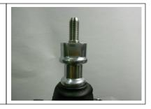
Apply ten full wraps of ½" wide Teflon thread tape on the threaded handle. Leave approximately 3/8" of exposed threads above the tape as shown in picture.
