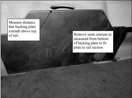
17. Place body brace backing plate on rail as shown with bottom of bracket on top of lower frame flange. It will need to be fitted to top section of rail. Measure how high it is above cutoff rail at top and remove this amount from bottom edge of plate.
