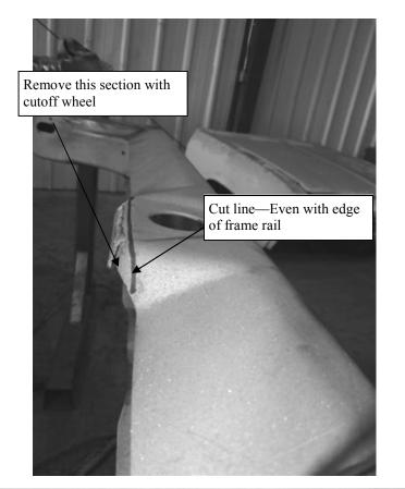
16. Cut section off top of rail at center body mount as shown in picture
