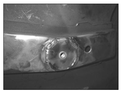
13. Clean floor brace so that clean bare metal is exposed and attach plate with threaded insert to floor brace as shown. The threaded insert will stick up into the floor brace
