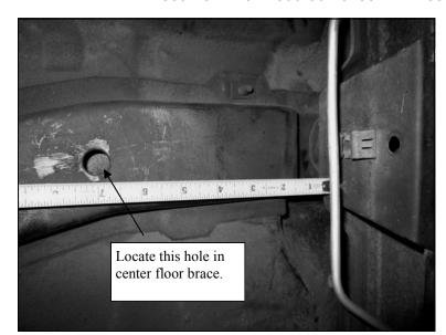
12.Locate hole in center floor support as shown. If hole does not exist skip to step 14 and hole will be added at a later time.
