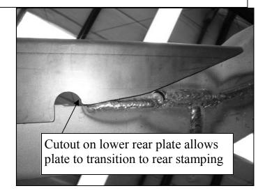
Lower plate overlaps bottom of c-section. Bottom of lower plate is parallel with lower edge of frame bracket.
