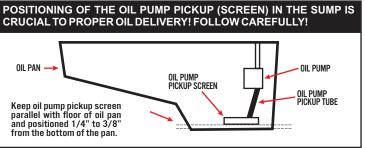
the distance between the oil pump pickup screen and the pan floor. The clearance <u>MUST</u> be between 1/4" - 3/8" with the <u>Hamburger's oil pan gasket installed</u>. If you are using a high volume pump, you may need to modify the pickup. For #3080 and #3090 Ford oil pans, see instruction sheet supplement.
