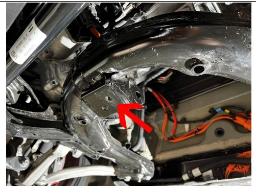
3. Install the provided bracket onto the mounting point located in the center of the subframe.
