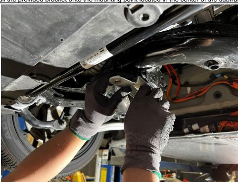
4. Position the bracket as shown with the threaded side facing the front of the vehicle. Secure the bracket to the subframe using one of the included M6 screws.
