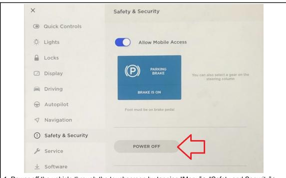
1. Power off the vehicle through the touchscreen by tapping "Menu" > "Safety and Security" > "POWER OFF".
