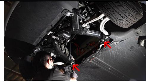
5. Install the M10 coupling nuts onto the large studs at the rear of the subframe. Use a 17mm socket and torque wrench to tighten to 35 ft-lb.
