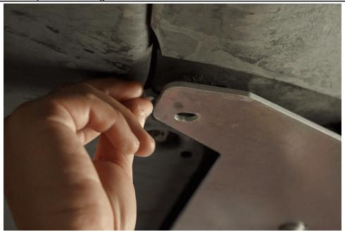
6. Add the provided spacers on the two corner of the plate near the battery
