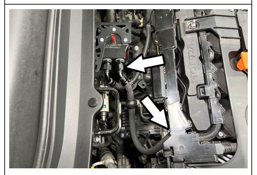
14. Connect the hose to the valve cover then connect the fitting onto the oil catch can. Check that the position of the fitting sits nicely between the engine cover and fuel hose cover before fastening.
