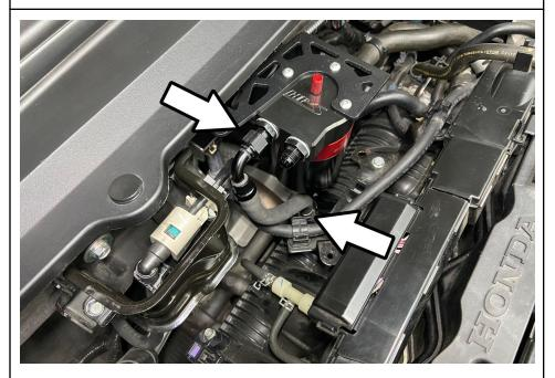
12. Connect the hose to the intake manifold before connecting the 90 degree AN fitting onto the port located closest to the firewall. Position the fitting to ensure at least 1/8" of clearance between the fitting and the fuel hard line, then secure the fitting.
