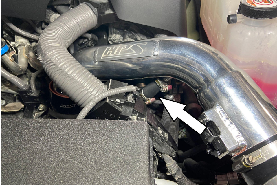
11. Connect and secure the longer leg of the hose assembly onto the valve cover and the shorter leg to the intake pipe.
